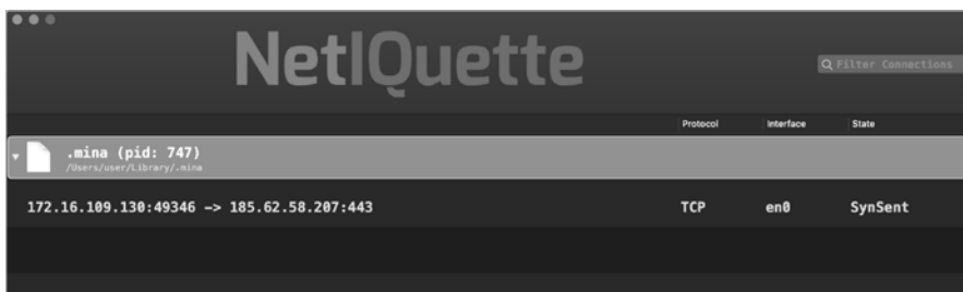
Figure 7-2: Using NetIQuette to uncover the address of a command and control server (Dacls)
